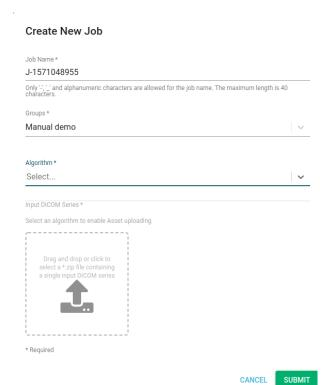
Insert the desired name (whitespaces not allowed, replace whitespaces with '-' and '\_'), select the algorithm and upload the images series (this needs to be a compressed file: \*.zip) and then click upload. Once you have uploaded an image series it can be processed again without uploading a second time using the prior uploads option.
